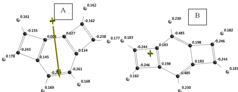
**Figure 7.** The ESP charges on atoms of the parent compounds considered.
