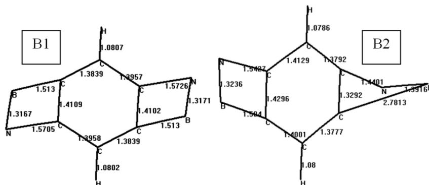
**Figure 6.** Calculated bond lengths/distances of B-series structures.
