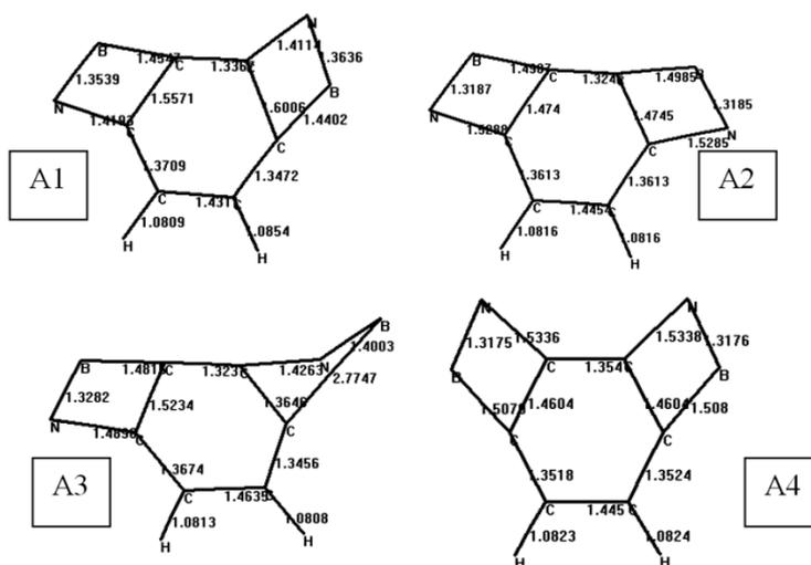
**Figure 5.** Calculated bond lengths/distances of A-series structures.
